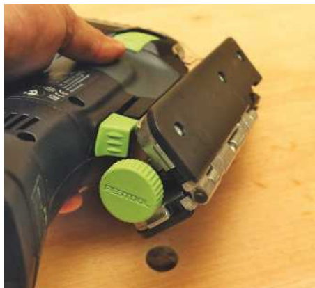
▲ ...or set to work the other way to sit into a rebate or cut to a straightedge
